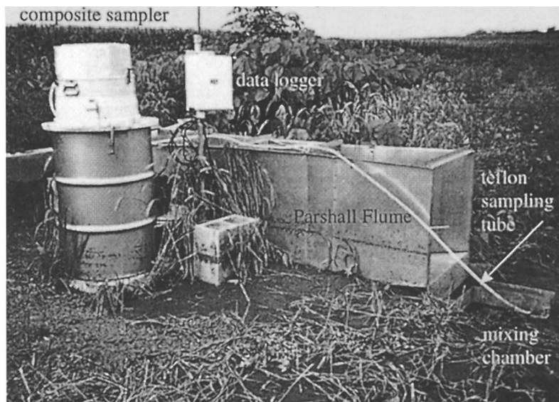
Figure 5. Secondary flume sampling station. Nested meso-plots have similar sampling and electronic equipment (with smaller trapezoidal flumes).
